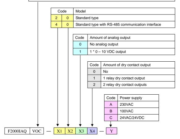
Example: F2000IAQ-VOC-2011 indicates the monitor can supply one analog output and one relay dry contact output.
